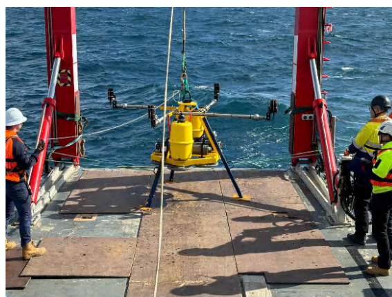
Floating microphones for marine animal monitoring in the South Taranaki Bight
